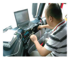
▲ CAN communication detection for a truck
